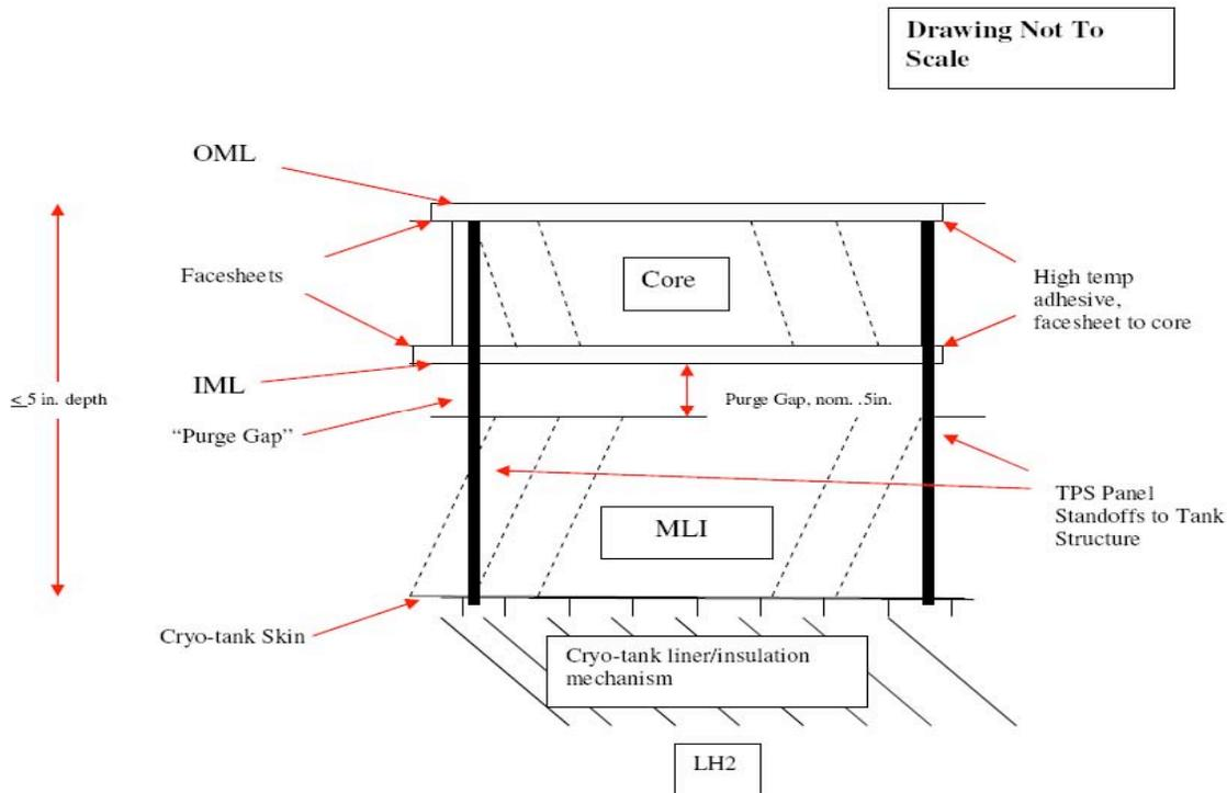
Figure 7. Schematic of concept 1 (with purge gap and standoff attachments).
