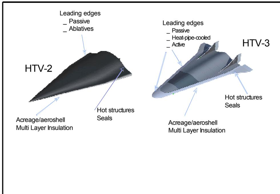
Figure 1. Materials on HTV-2 and HTV-3 requiring development.
