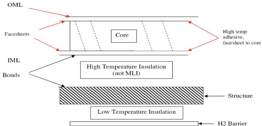
Figure 8. Schematic of concept 2 (without purge gap or standoff attachments).
