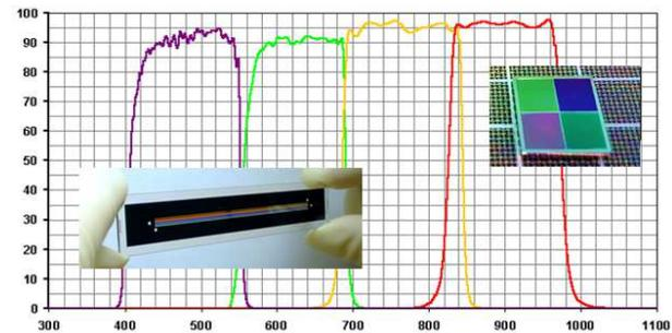
Figure 6: Reosc 2D structured high efficiency filters
