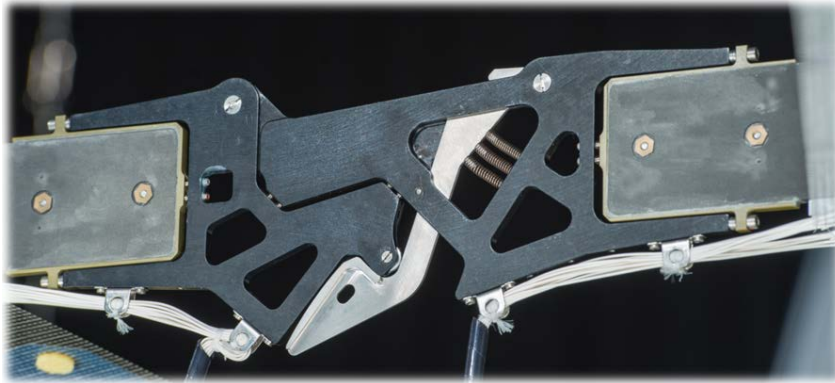
Figure 8. Folding and Latching Spar Joint Assembly Hardware
